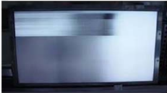
Horizontal Block Gate TAB IC Defect
