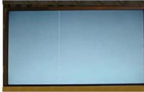
Vertical Line Source TAB IC Defect
