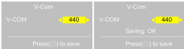
(Visual Adjust and control the Voltage level)
